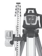
Make sure pad is level around entire circumference of pad and across centre using laser level.
